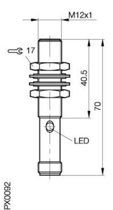
Inductive Sensors BES 516-207-S 27-E M12x1 x 70 normally-open Sn=2mm shielded
